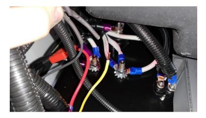
4. Cut the switch wire and strip back the sheath on both ends about 5" away from the 4-way connector.
