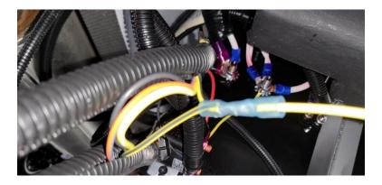
6. Butt connect the single ignition wire end to the other end of the spare 10" yellow wire.
