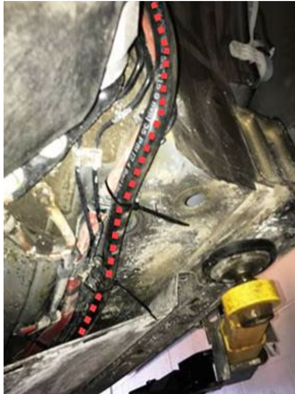
Figure 7. Where to zip tie the rubber hose to the battery cable.
