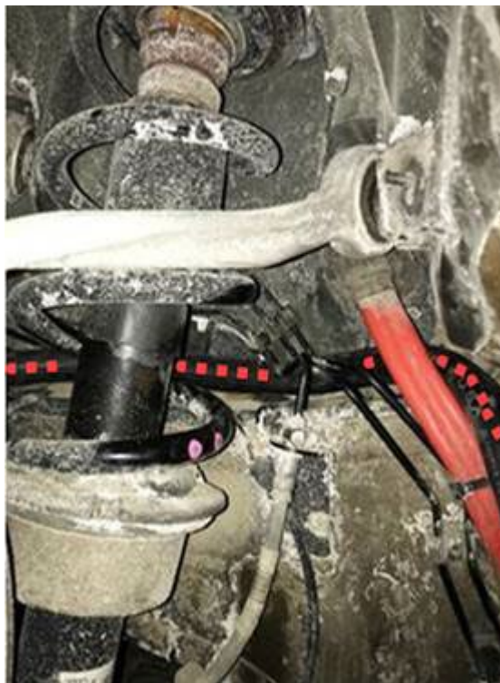
Figure 6. Routing the rubber hose.
