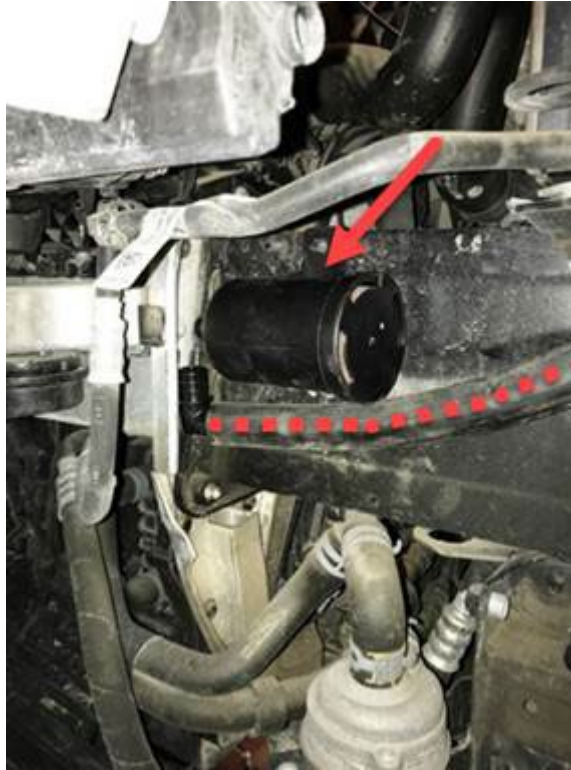
Figure 3. Installing the new NLVD filter.
