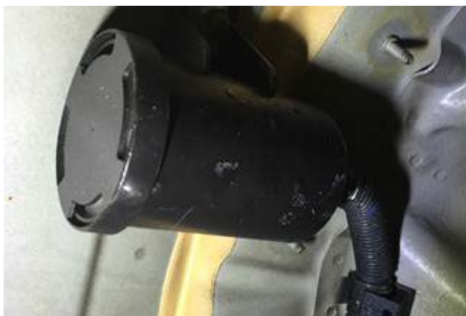
Figure 10. Remove original NVLD filter.
