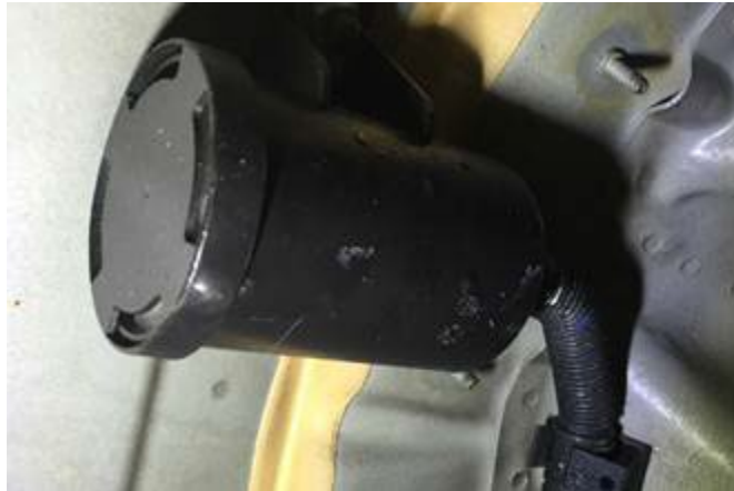
Figure 2. Ventilation tube of the EVAP canister.
