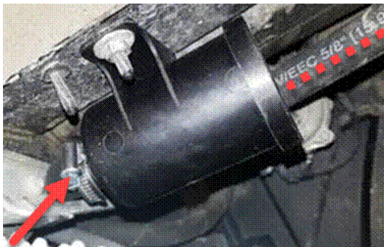
Figure 4. Connecting the NLVD filter.
