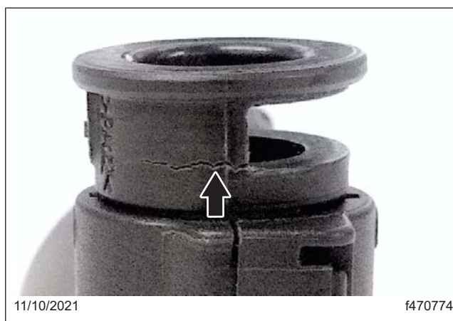
Fig. 1, Line Damage Resulting from Freezing DEF
