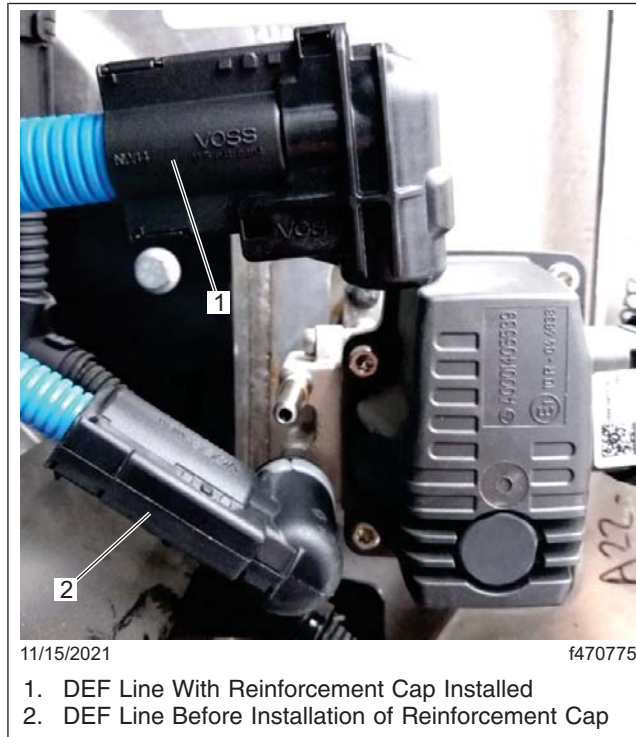
Fig. 2, Reinforcement Cap Installation
