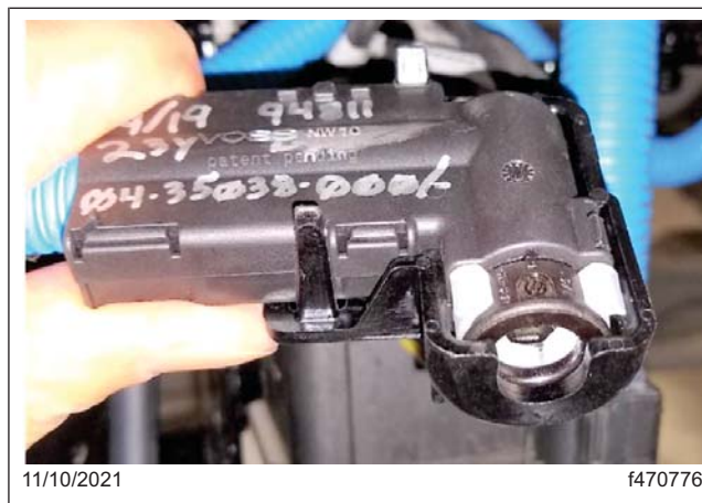
Fig. 3, Reinforcement Cap Installation
