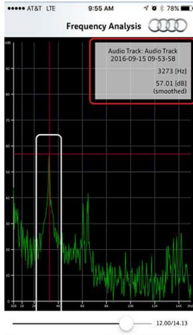
Figure 10. Typical brake squeal frequency recording.
