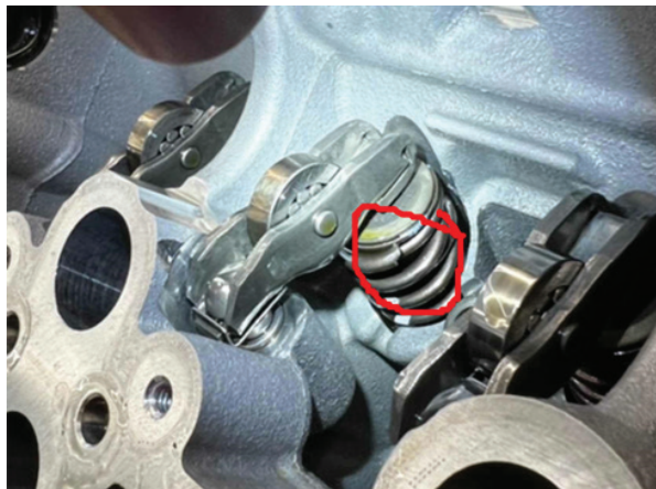
Figure 1 - Broken Valve Spring
