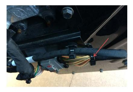
If the cable tie is found to be cutting into the wire insulation, remove the cable tie, wrap the exposed wires in harness tape and re-clip the harness securely.
