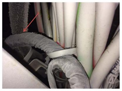
If the ACM harness is rubbing the air compressor discharge hose, make sure the harness is clipped to the airline bundle securely as shown above. Attach a separator tie between the harness and the discharge hose to keep the two apart.
