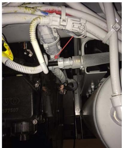
If the harness is contacting the DEF lines, attach a separator tie between the harness and the lines to keep them apart.
