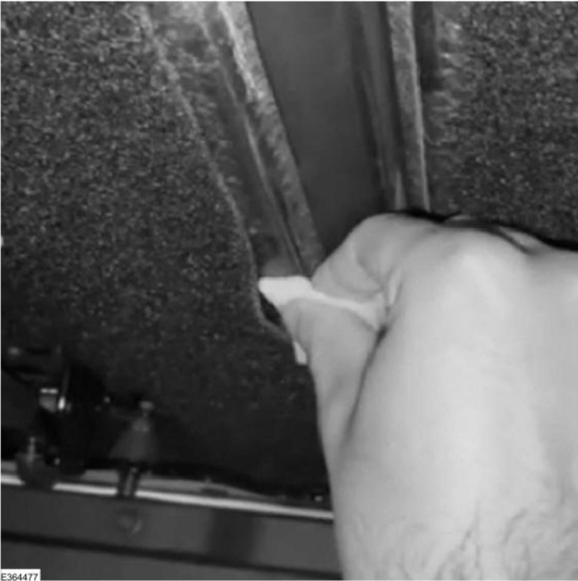
3. Press the headliner back into position and hold for at least 40 seconds too allow the adhesive to set. (Figure 3)
