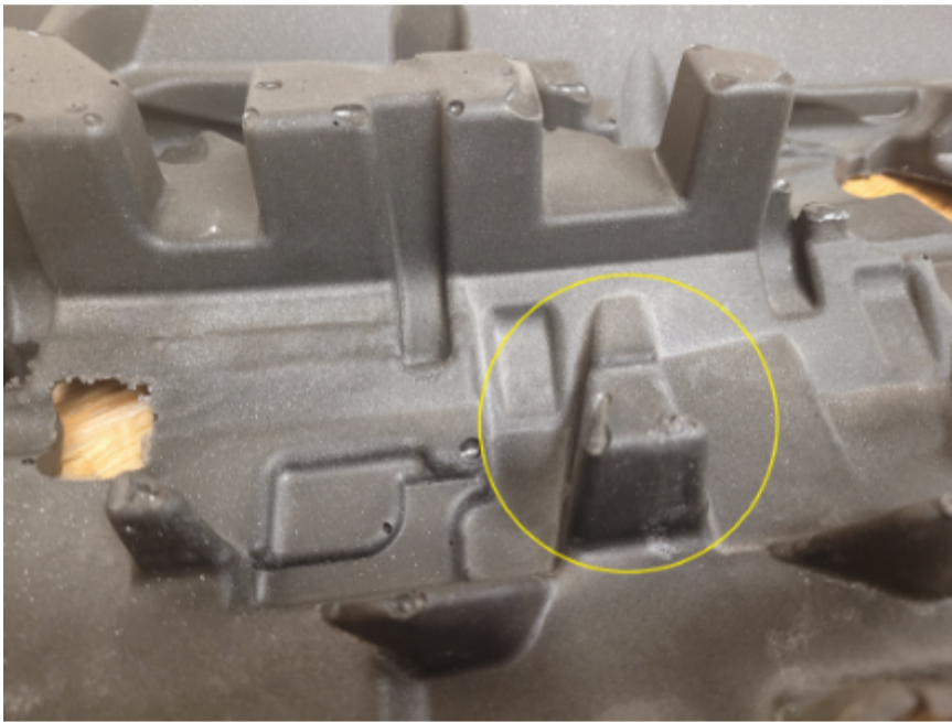
Cut the standoff flush with the surrounding area.
