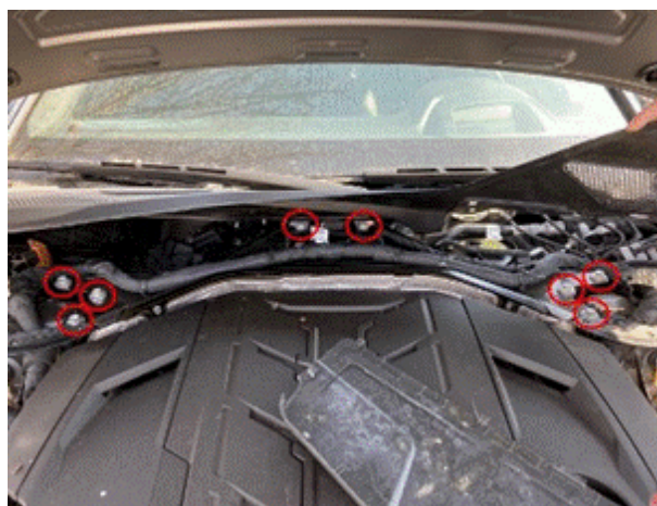
Figure 1. The strut brace bolts that are found loose after visual inspection.
