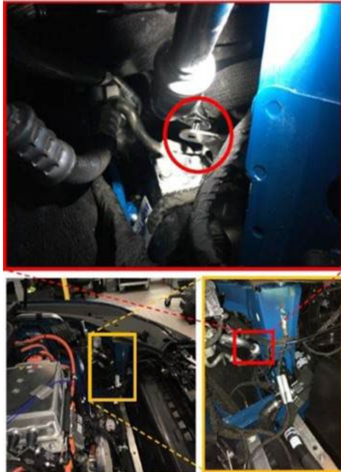
Figure 4. The area in the motor bay where contacting lines are located.
