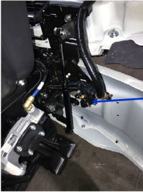
Charge Air Cooler (CAC), Radiator and AC Condenser Lines and hoses for these components Supplied by Hino
