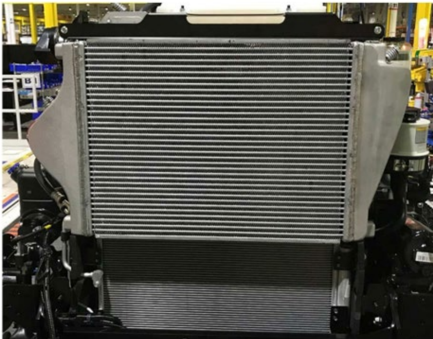
Charge Air Cooler (CAC), Radiator and AC Condenser Lines and hoses for these components Supplied by Hino
