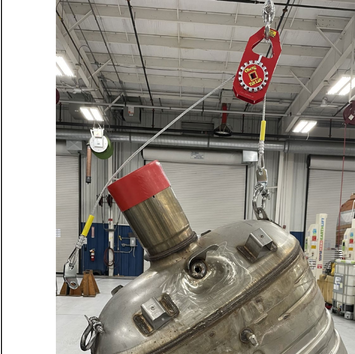
Oberg tilt lift 2,000 lbs. Capacity – special lifting tool available in Service Centers use with half-inch ratchet or half-inch breaker bar
