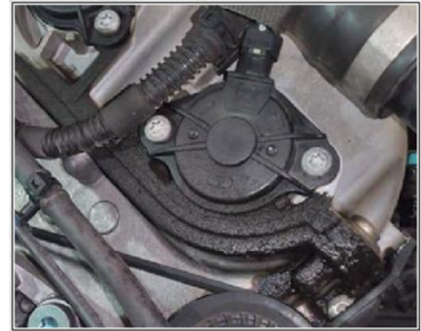
Sample illustration: Oil leak in the camshaft phaser
