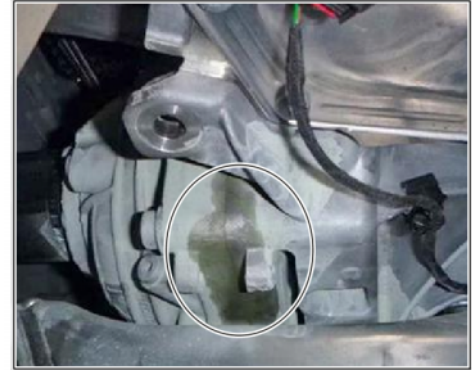
Example of oil residues on front-axle drive
