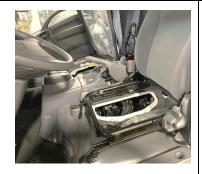
**Driver Front Seat (Access** the front of the engine, power steering pump, vacuum pump)
