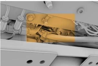
• If the clearance is approximately 1 inch (2.5 cm) or more, the correct bracket is already installed. No additional work is required. Reinstall all components that were removed for access and replace all non-reusable components.
