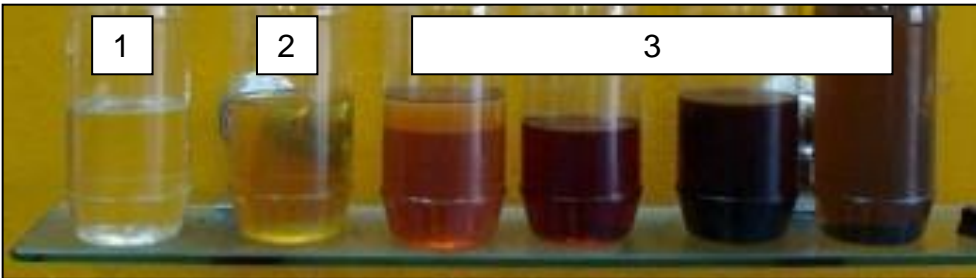
Figure 3: Refrigerant oil color overview
