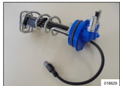
Figure 1:-DEF tank sensor unit (6th generation)
