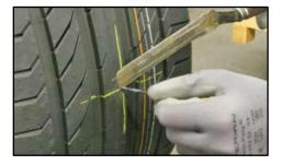
9. Apply tire cement glue over the patch surface area where foam patch was cut out and removed.
