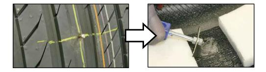
6. Apply cement glue to the tire puncture area and plug patch.
