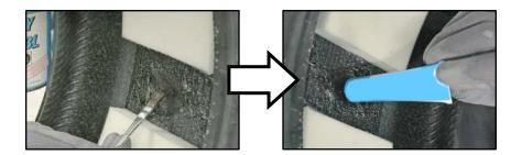
7. Install the plug patch until firmly flat inside the tire and roll out patch surface to promote adhesion.
