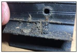
Figure 5. Example of Debris on Drain Hole
