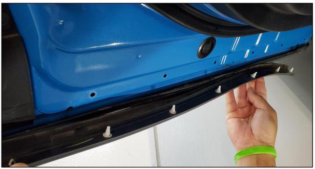
8. Ensure the cut window on the weatherstrip molding and the drain hole align properly.
