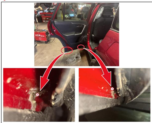
Wax-type Substance Blocking the Door Drain Holes
