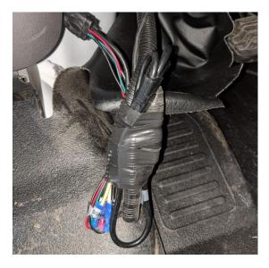
5. The picture below is how the connections look when the splitter is installed correctly. Once installation is complete re-tape the wires into a bundle and put bundle back up behind the plastic and reinstall plastic cover.
