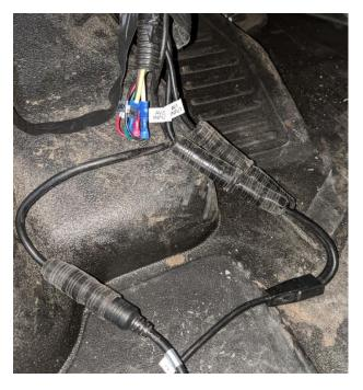
6. Test for correct function by turning on the ignition and then hitting the button on the monitor. It should turn on and display the camera image if installed correctly. Also test by putting the coach into reverse and ensuring camera is operational.
