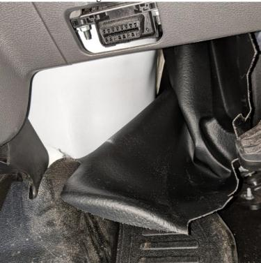
4. Pull the bundle down for better access. Remove electrical tape from bundle and install splitter
