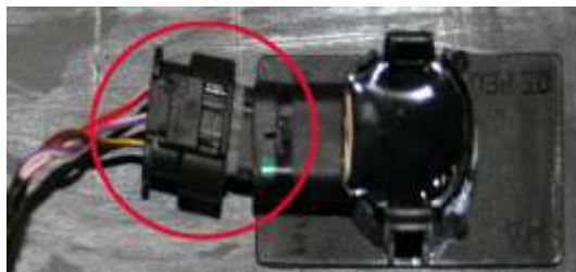
Figure 7. Example of a parking aid sensor connector that is not seated correctly.
