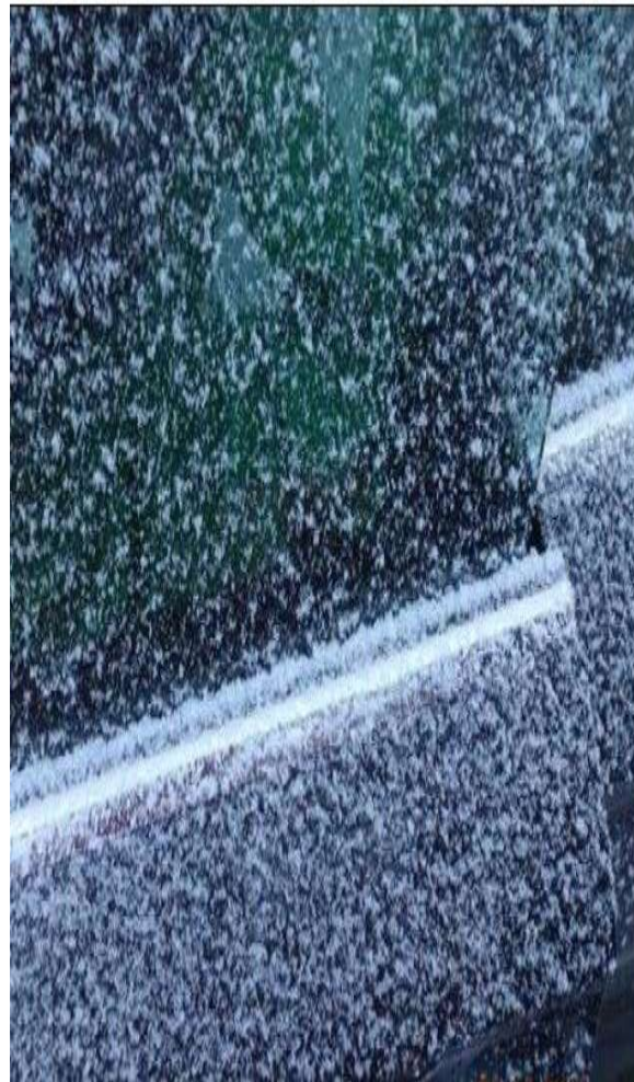
Figure 1. Snow and ice build-up on window and window slot seal surfaces.
