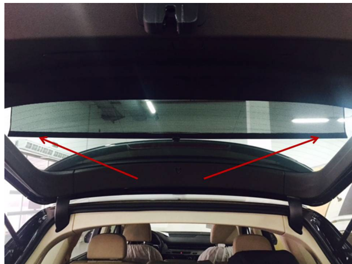
Figure 1. Rear window sunshade has lost its tension and does not fully retract.
