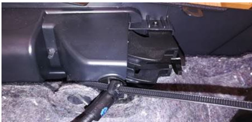
Figure 2. The Bowden cable; reinstalled and secured with a tie wrap.
