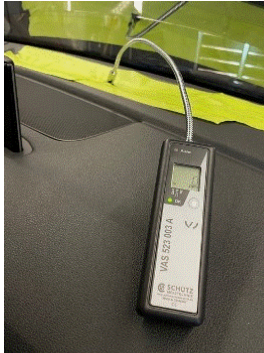
Figure 6. VAS 523003A gas leak detector in place in the defroster outlet.
