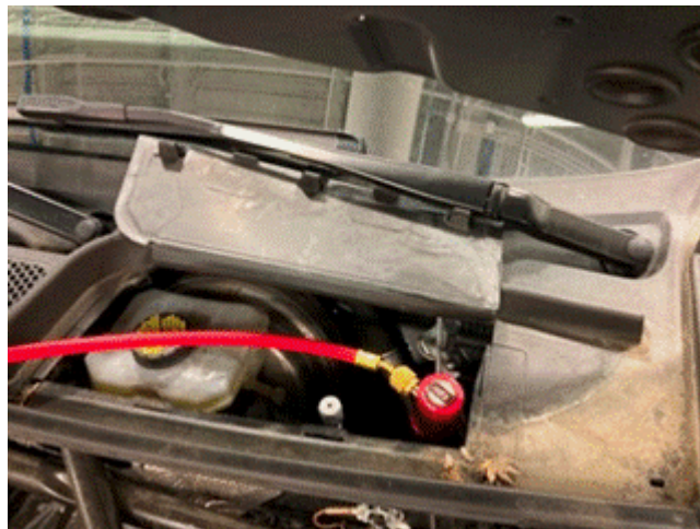
Figure 4. NITROKITG high side snap coupler connected to the high side service port.
