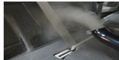
Figure 5. Correct positioning of the outlet tube on a Q7.
