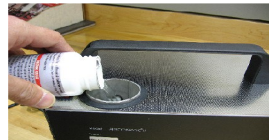
Figure 2. Pouring the treatment into the filling chamber.
