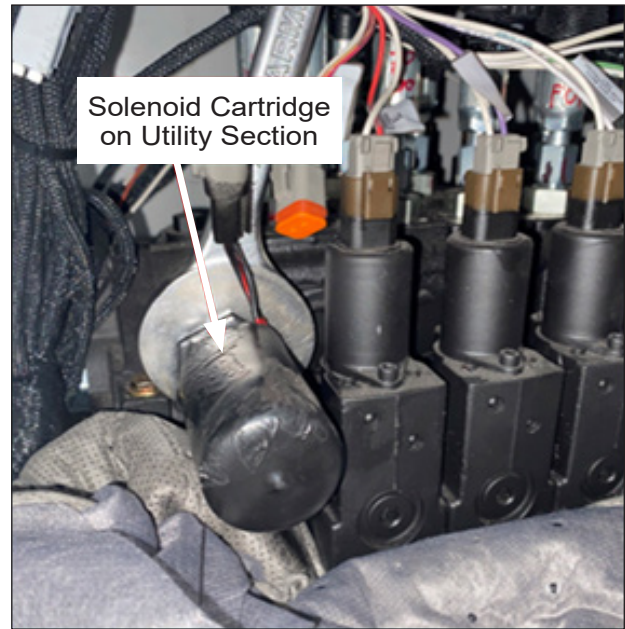
Figure 3 — Valve with Solenoid Cartridge Installed
