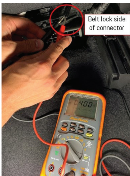
Figure 3: Resistance check for (4a)
