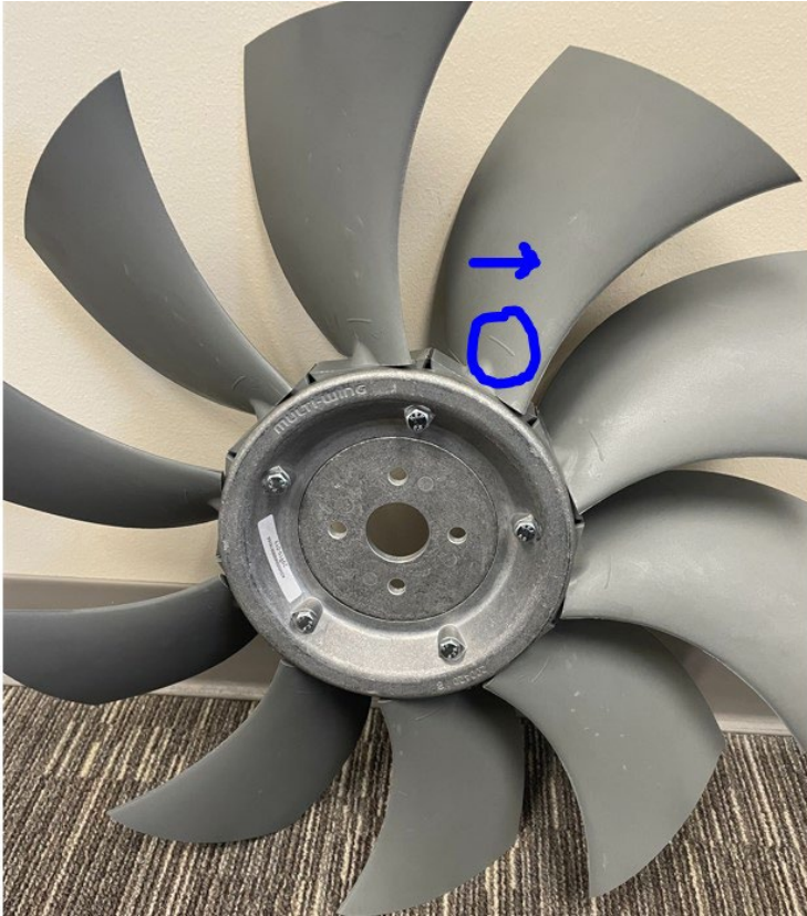
Wrong fan – Arrow points to right .
