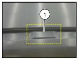
e. Apply adhesive around each clip (1) (on the yellow rectangular areas) after installing "Clip A's" on the vehicle.
