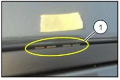
This is caused by the gap between the roof molding attachment clips and the roof panel not being wide enough to allow paint to be appropriately applied to the roof panel. To eliminate this concern, the shape of the roof molding clip has been changed to enable paint application between the clip's rib and roof during the manufacturing process. Customers having this concern should have their vehicle repaired using the following repair procedure.
