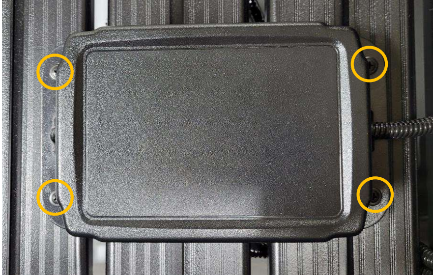
Figure 4 Remove (4) screws securing box to roof rack
