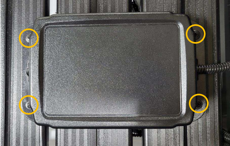
Figure 10 Reinstall (4) screws securing box to roof rack
