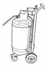
Use the coolant extractor to fill the system with approved coolant per specifications.
