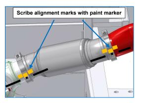
That Flexible pipe is positioned so the flanges are sitting flat against each other. Any misalignment of the flanges at re-installation will cause the gasket to be unevenly compressed and make the joint prone to leakage.
