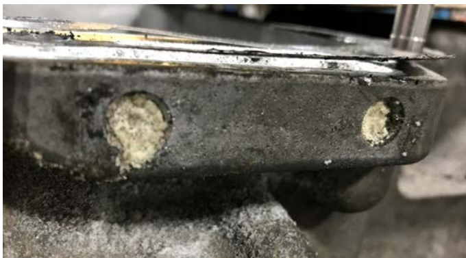
Clogged vent ports
