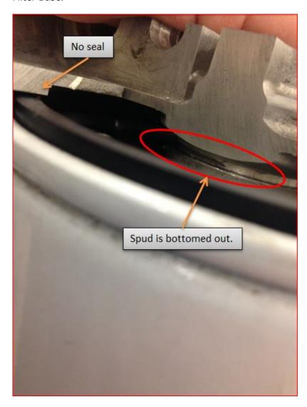
For additional information on the correct application Volvo / Mack Fuel Filters refer to CBR solution:
