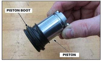
Next, set the piston into the caliper and work the piston boot flange into the caliper groove with a blunt tipped tool until it is fully seated.
