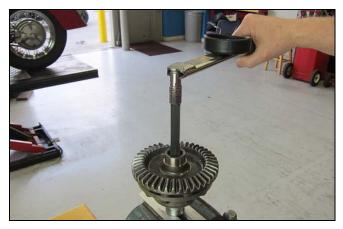
If the slip torque is out of specification, disassemble the differential and perform the components inspection as the differential may be faulty.
