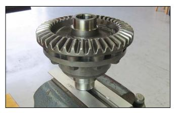
4. Install the "B" side of the second tool into the other side of the differential as shown.
