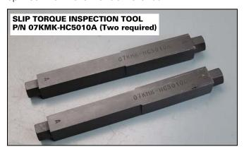
Here's how to set-up the tools and measure the slip torque of a TRX front differential:
