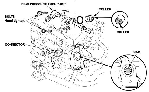
18. Install the roller and the high pressure fuel pump. Install the bolts loosely by hand in an alternate pattern. Connect the connector.
