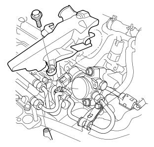
5. Remove the quick-connect fitting cover.
