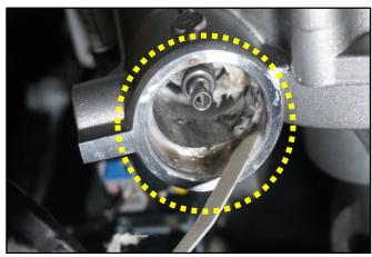
15. Remove the bolt (H) from the MDPS small bearing mounting tool. This bolt will be used to locate the tool on the MDPS housing.
