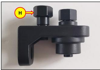
16. Insert the new, small bearing into the bearing holder.
