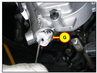
13. Use the MDPS small bearing removal tool, to remove and discard the bearing.
