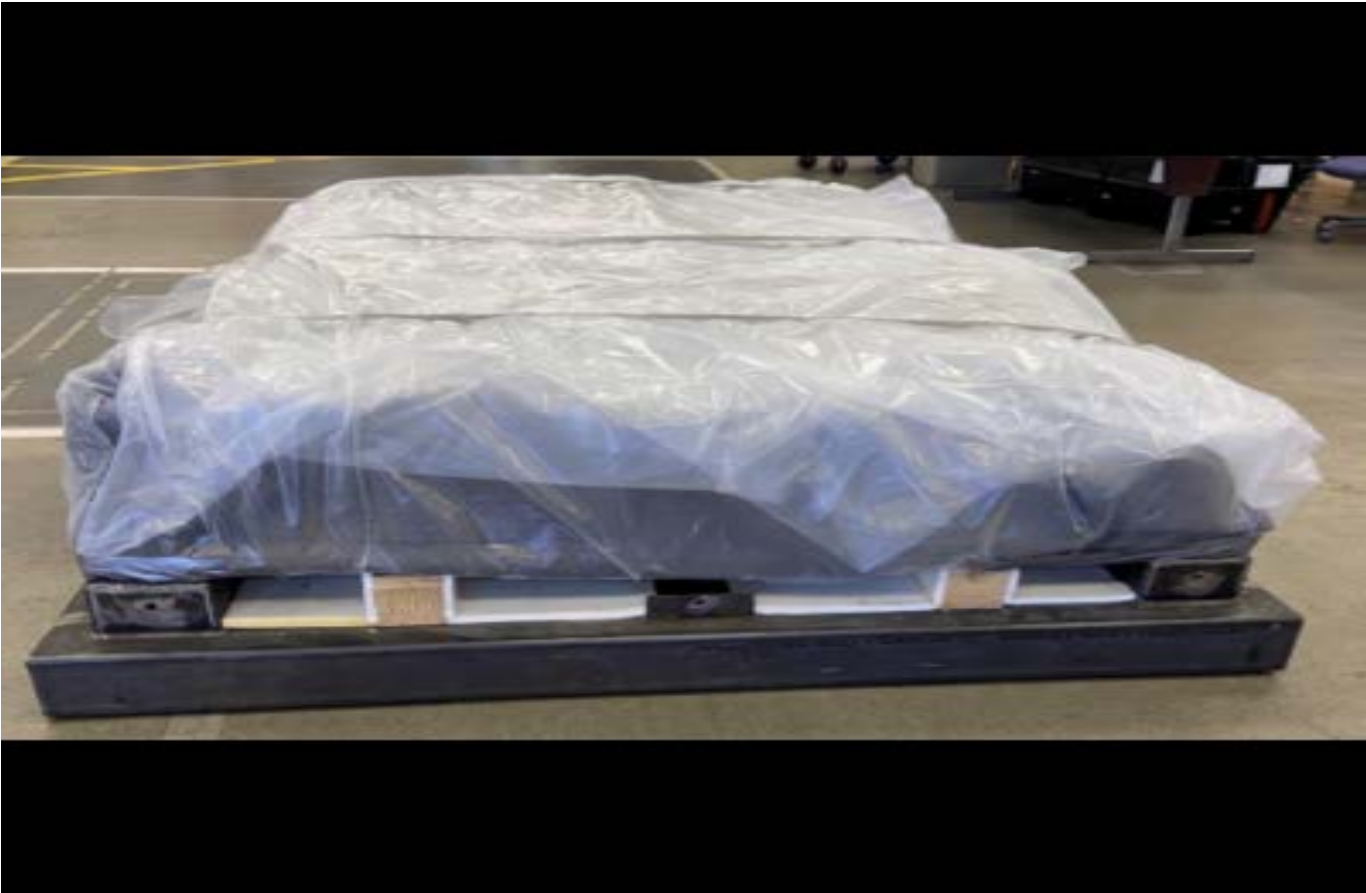
28. Completed wrapped battery.
