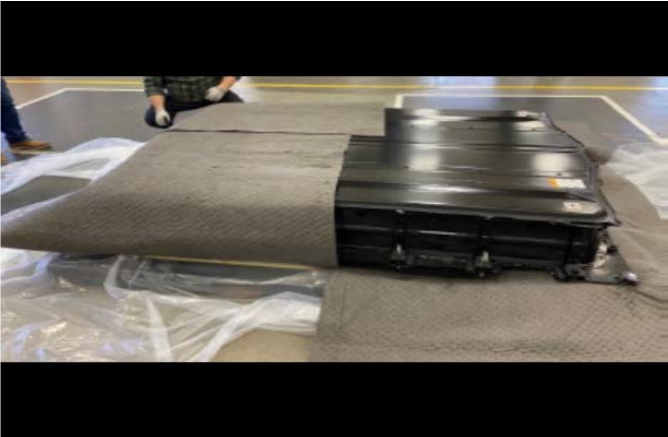
20. Wrap battery with first absorbent pads as shown above.
