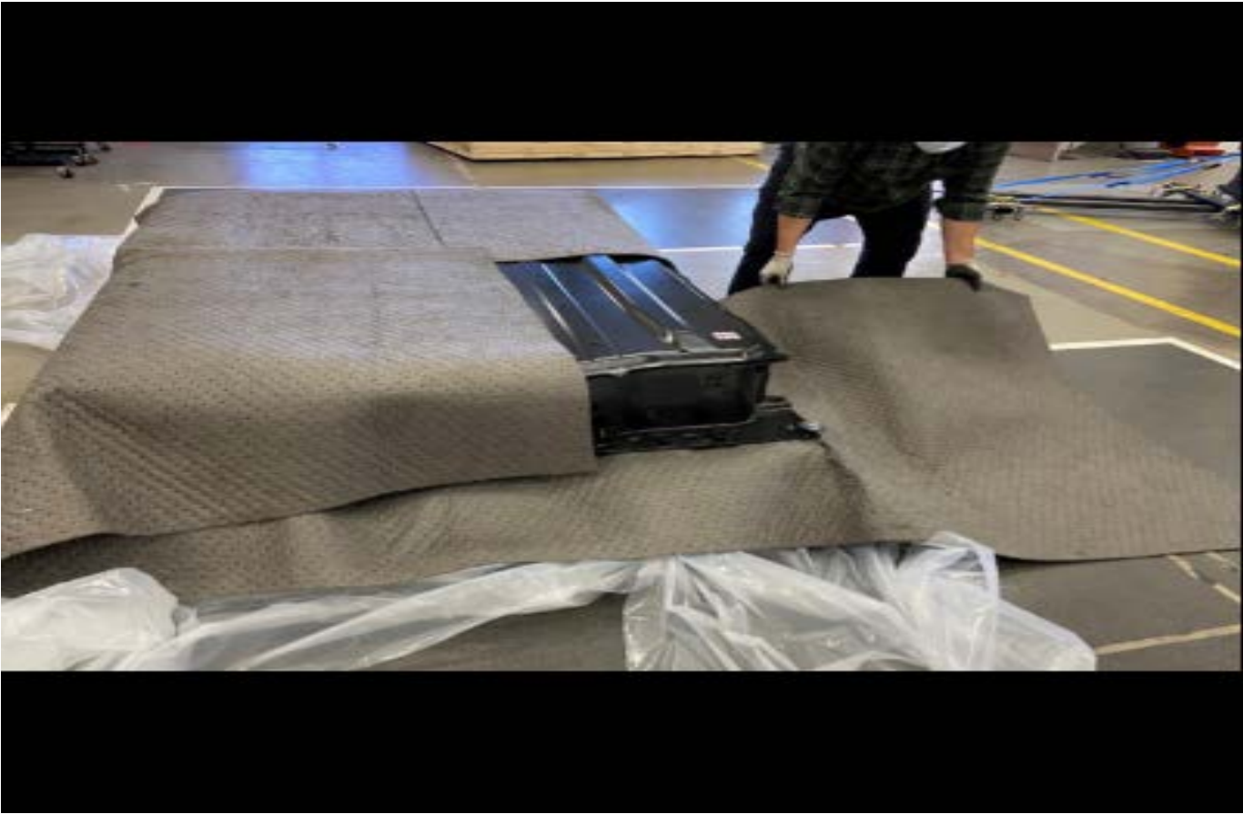
21. Repeat with second absorbent pad.
