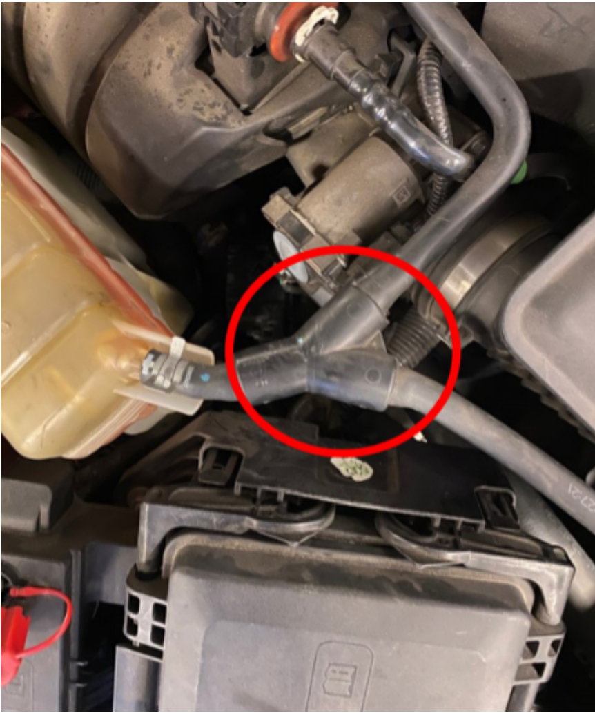
Coolant "Y" Hose Leak
