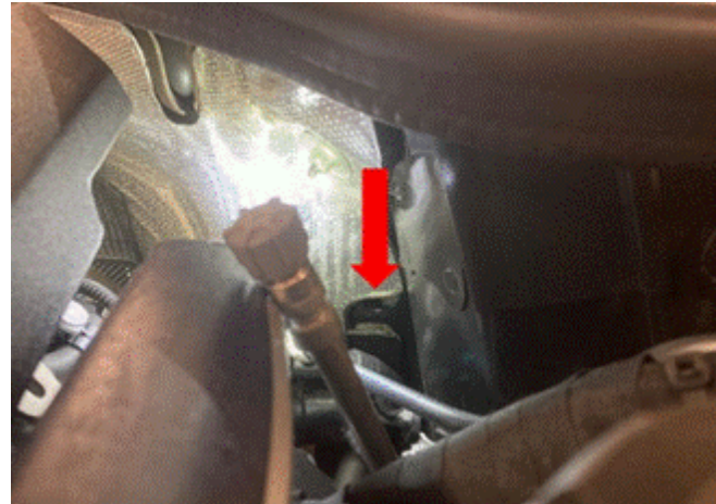
Figure 3. Body plug 4N0 811 817 A installation location.
