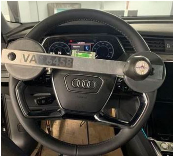
Figure 1. VAS 6458 installed with steering wheel off-center.
