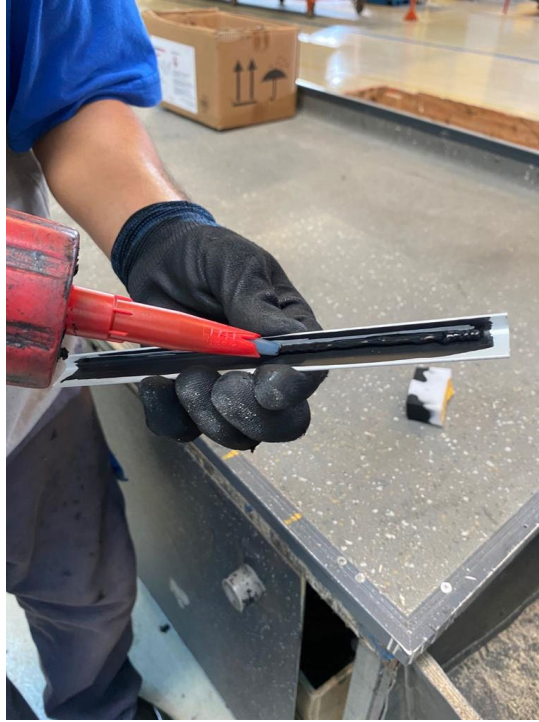
Figure.6 Application of the sealer to the L profile
