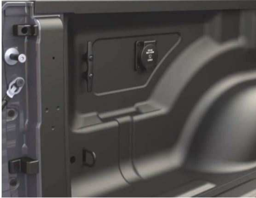
Fig. 5 RAM Bed Mounted AC power outlet
