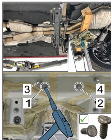
Removing fastening bolts
