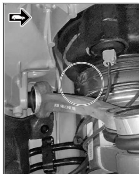
Damage to front right air-spring strut
