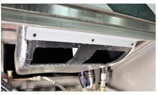
Inside the vehicle, install the # 454469 and the # 454466 supports on each side of the duct opening. Use 4 supplied # 500957 screws for each support, two on the top and two on the side of the duct.
