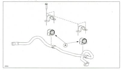
NOTE: To prevent noise from occurring, never apply any type of grease or lubrication to the front or rear stabilizer bushings.
